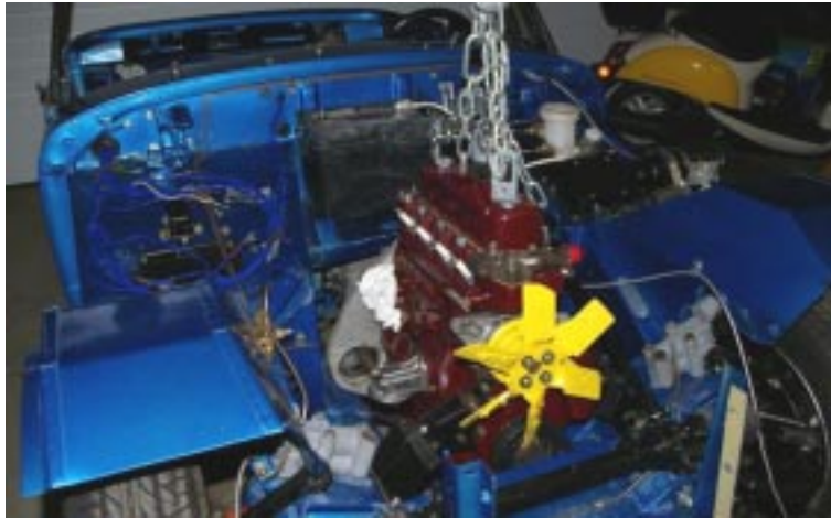
Successful installation of the Datsun 5-speed and 1275 engine.
