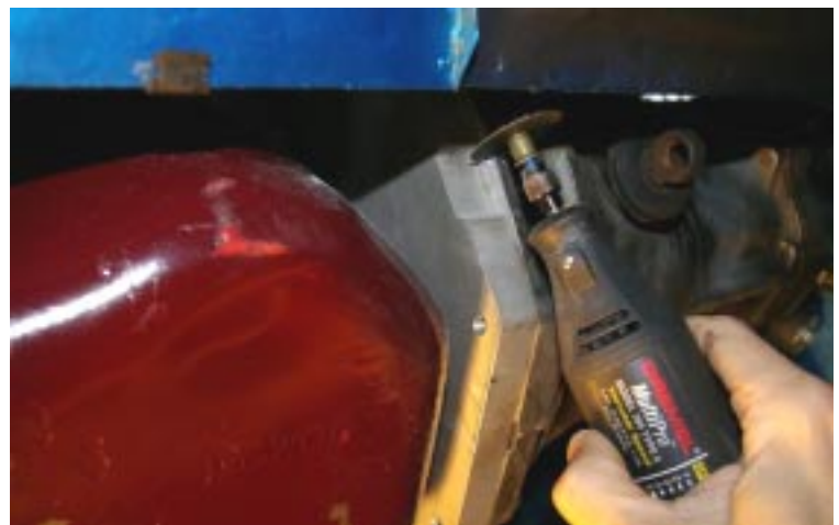
Dremel cut-off wheel modification for slave cylinder.
