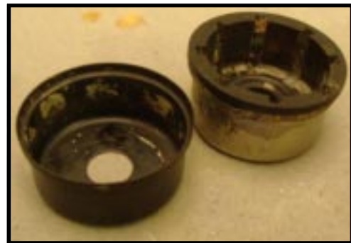
Left—what came out of my booster. Just the metal cup retainer. Right—the vacuum seal as it should be.
