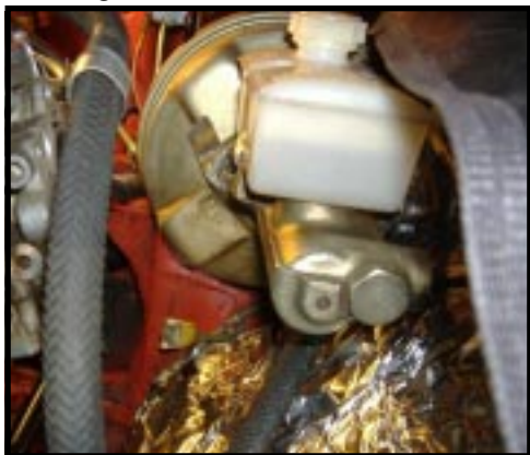
The brake master and my aluminum foil protection lining I put in place to protect the engine bay paint.
