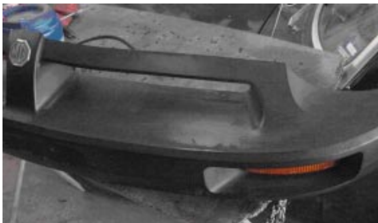
Before repairs. Notice the dull, crazed finish. Home restorers should remove bumpers first.
