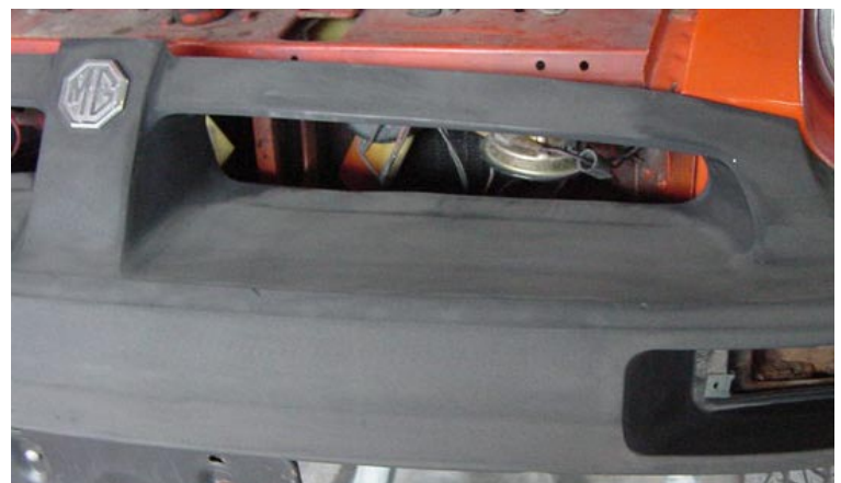
Bumper after cleaning with wax & grease remover and initial sanding.
